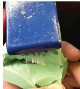
Not Dipped - Sticking to Mould
